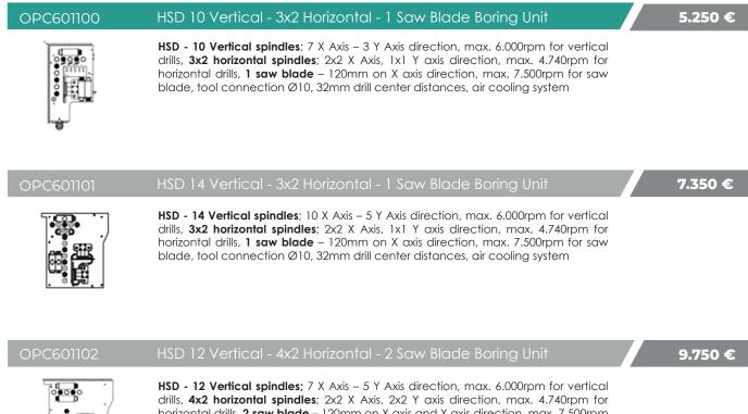
horizontal drills, 2 saw blade – 120mm on X axis and Y axis direction, max. 7.500rpm for saw blade, tool connection Ø10, 32mm drill center distances, air cooling system
