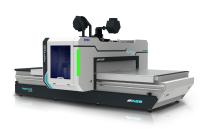
Working Dimensions 1300 x 2500 mm / Z Axis Stroke 200 mm
